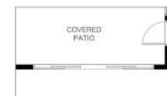
② EXTERNAL SLIDING DOOR TO COVERED PATIO
